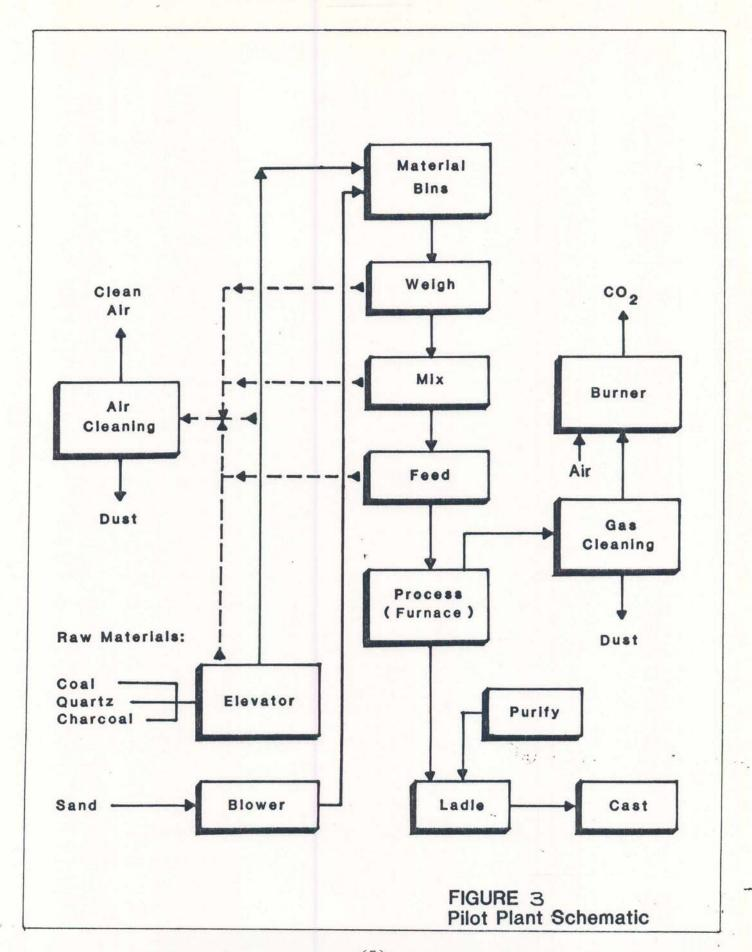
carbon source. The silicon product produced by the reduction reaction would be tapped to a ladle where it would be purified by oxidation, using an oxygen gas blowing operation. After purification the silicon product would be cast and allowed to solidify. For shipment, the silicon casts would be crushed to facilitate transport.
