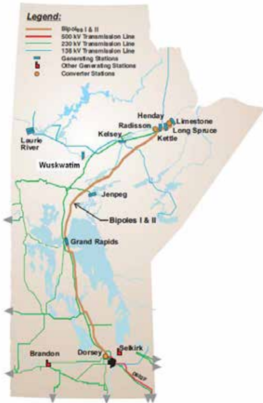
Fig. 4.2 Manitoba Hydro's northern generating stations and major transmission lines
