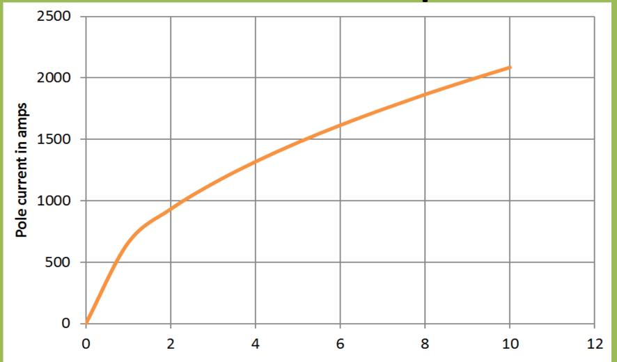
Temperature in Degrees Celsius of each pole sub-conductor above ambient for Bipoles I and II
