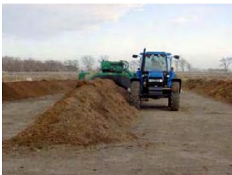
Figure 6.9 Windrows with mechanical turning (Freeze et al.)
