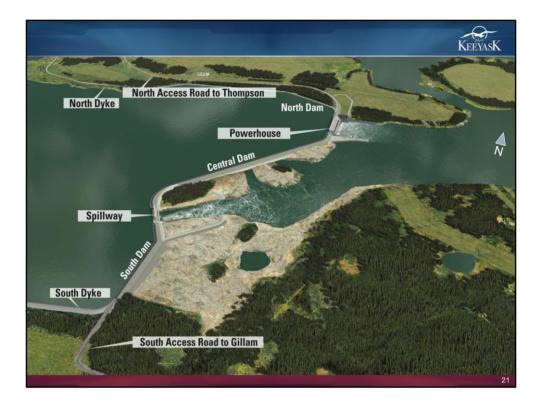
The spillway will manage surplus river flows, and the dams and dykes will contain the reservoir created upstream of the principal structures. The reservoir level will operate within a narrow one-metre range. The full supply level will be 159 metres and the minimum operating level will be 158 metres.
