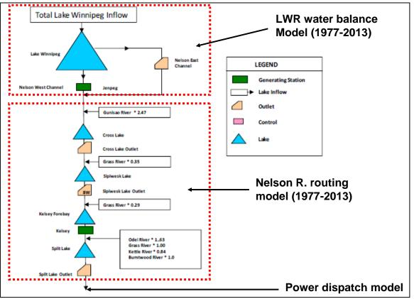
Figure 2.1: Domains and components of MH Lake Winnipeg and Nelson River spreadsheet Routing Models
