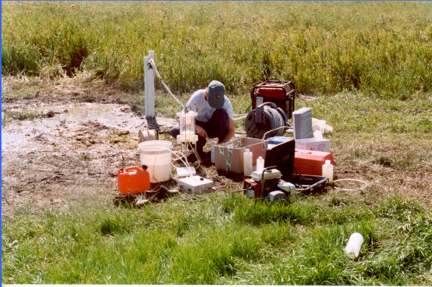
Collecting samples for chemical analyses of groundwater
