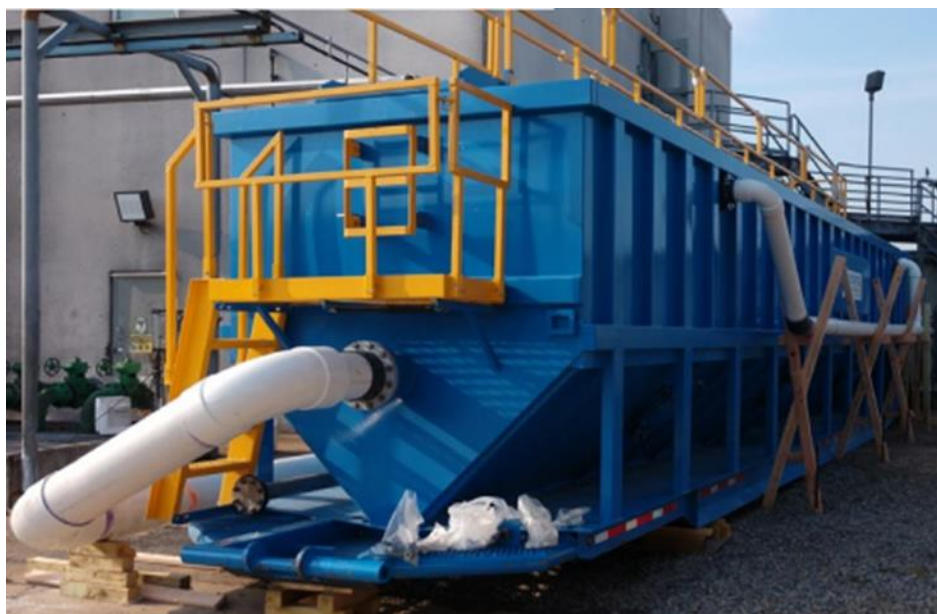
Figure 4-3: Mobile Clarifier Units by Monroe Environmental
