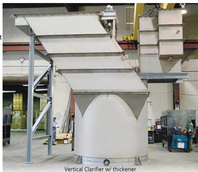
Figure 4-4: Typical Lamella Clarifier System (Figure Courtesy of Monroe Environmental)
